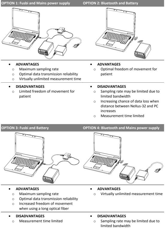
Increasing chance of data loss when distance between NeXus-32 and PC increases.
