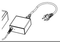
Check that the power supply is labeled as 'SUP3'. Connect the mains cable to the power supply and the other side into a well-grounded power outlet. The LED on the power supply will light up green.
