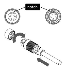
Connect the power supply cable into the power supply socket on the front of the device (POWER).
