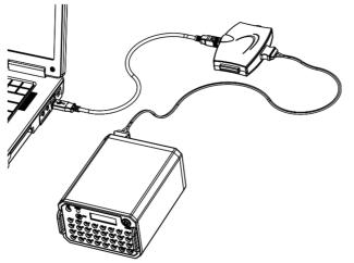
1. Connect the optical fiber to the input of the Fusbi and the other end to the fiber connector on the NeXus-32. It does not make a difference which connector goes where.
