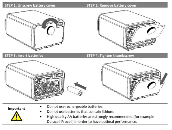
Please note that it is not required to use all free battery slots in order to power the device. NeXus-32 devices also run on 6 AA batteries (in one row) instead of 12.
