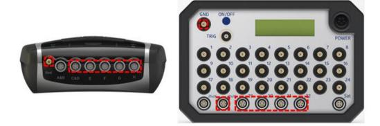
Connect the EXG Ground to the Ground (Gnd) of the NeXus.
