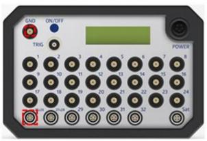
Sensors can be disconnected by pulling the silver ribbed part of the connector backward.
