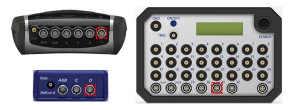
Sensors can be disconnected by pulling the silver ribbed part of the connector backward.
