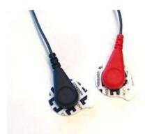
Place the red (positive) and black (negative) electrodes on to the skin at the position of interest. Make sure the electrodes at the muscle of interest are placed parallel to the muscle fibers. The orientation of the positive and negative snap-on is not critical, they can be mutually swapped. Usually the electrodes are placed right next to each other.
