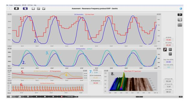
The following is displayed in the therapist screen: Heart Rate (1); Respiration wave (2); Pacer (3); Skin Conductance (4); Temperature (5); Raw ECG or BVP signal (6); EMG amplitude (7); Spectral Display (8).
