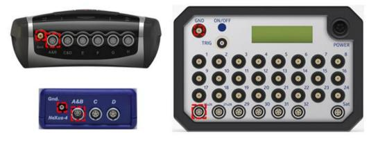
Snap the electrodes on to the black and red snap on of **pair two** of the EXG Sensor. The use of high quality electrodes like ECG Meditrace or ARBO electrodes is recommended.
